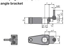
Special clamping arm 1. Connecting dimensions
