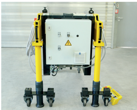
Option: The control is directly mounted to the console, console and control can be completely removed.
