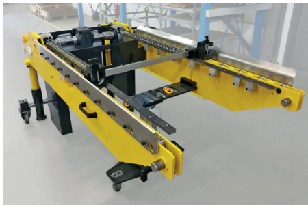
View of pull-push chain and die adapter
