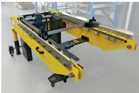
View of pull-push chain and die adapter
