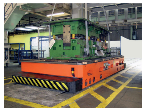
Transport cart, movable on rails
