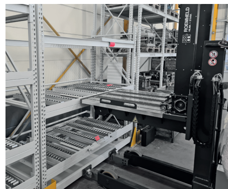
Die changing cart RWA 4000 with docking bar and pull-push chain
