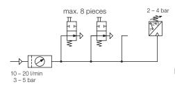
For the evaluation of the pressure built-up standard electro-pneumatic pressure switches can be used.
