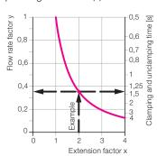
Adm. flow rate and clamping time as a function of the clamping arm extension
