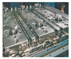
Swing sink clamps in a double-column press The tie rod is extended (swing position). Die positioning is made by lateral stops. Easy feeding of dies by hydraulic roller bars installed in the T-slots.
