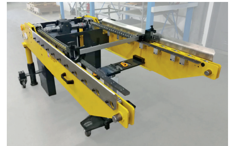
View of pull-push chain and die adapter
