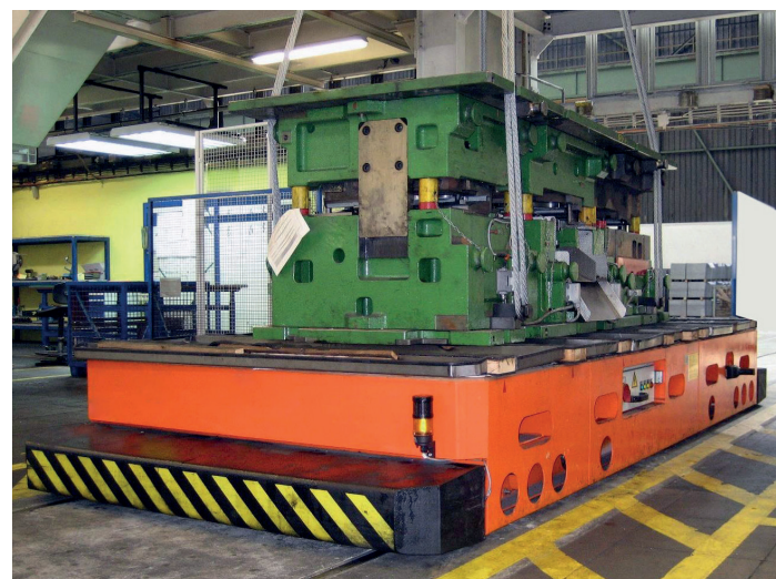
Transport cart, movable on round rails
