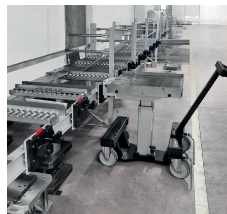
Rack system with docking hooks and die changing cart RW 500
