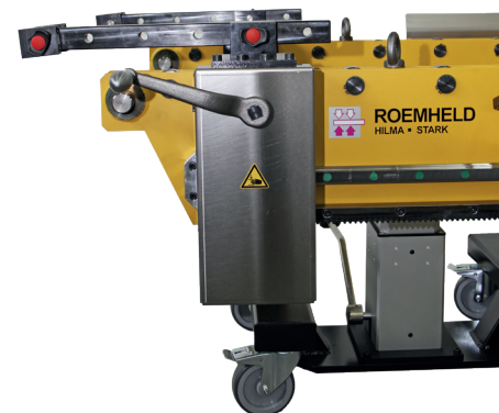
Die changing console with crank handle and transmission gearing
