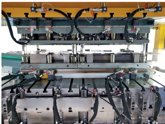
Sliding clamps with T-slot adapter in the press bed and ram
