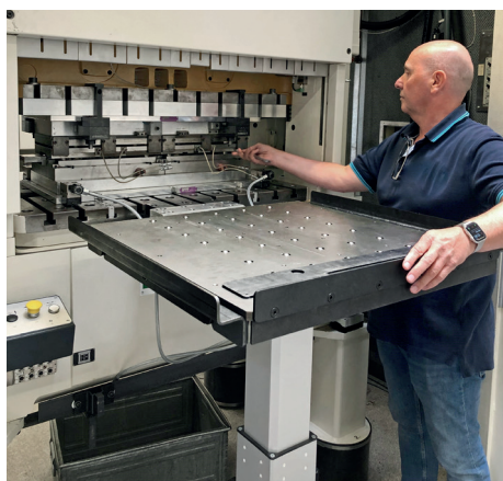
Application: die changing cart RW 500 with ball table on a Bruderer punching machine.
