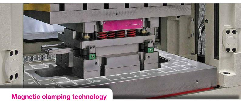
R-MAG magnetic clamping plates and systems for injection moulding machines, forming presses for sheet metal forming, rubber presses and mould carriers or die casting machines
