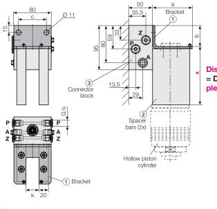
Distance dimension "x" = Dimension "f" – ½ stroke please specify when ordering Hydraulic circuit diagram
