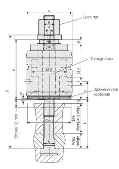
Freely adjustable and flexible adaptation to suit varying heights of clamping edges of the dies by quick and easy adjustment of the tie rod by means of a lock nut.
